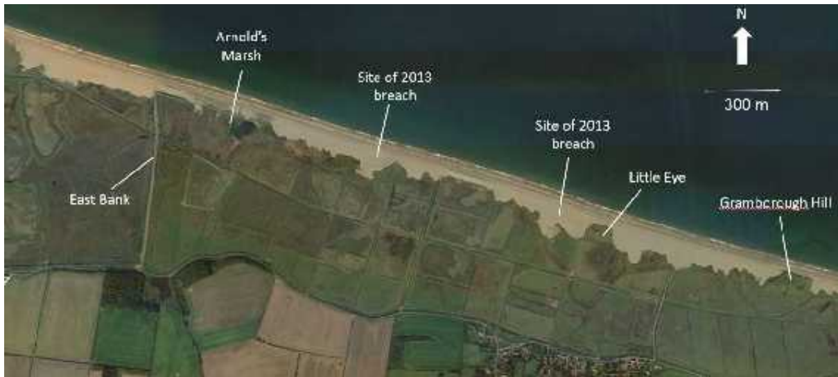
Figure 3-20. Salthouse Marshes between the Cley East Bank and Gramborough Hill showing location of geomorphic features associated with the 2007 and 2013 storm surges. Google Earth image 24 th September 2017 (Andrews, 2020)
